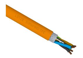
LUTZE Silflex flexible servo cable, shielded, 4 conductors (includes ground), 10 AWG, bare copper, (1) shielded 18 AWG twisted pair, PVC/Nylon conductor insulation material, brown, black, blue and green/yellow ground, TPE jacket, orange, cut to length.
