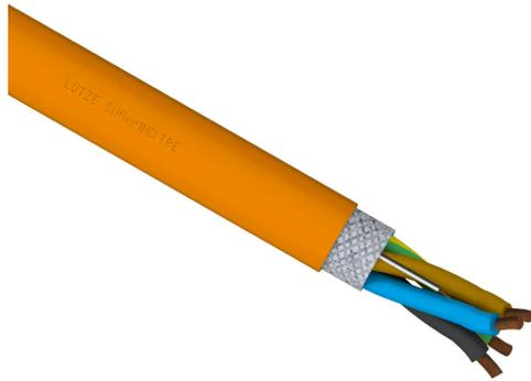
LUTZE Silflex flexible servo cable, shielded, 4 conductors (includes ground), 6 AWG, bare copper, (1) shielded 18 AWG twisted pair, PVC/Nylon conductor insulation material, brown, black, blue and green/yellow ground, TPE jacket, orange, cut to length.
