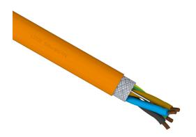
LUTZE Silflex flexible servo cable, shielded, 4 conductors (includes ground), 4 AWG, bare copper, (1) shielded 16 AWG twisted pair, PVC/Nylon conductor insulation material, brown, black, blue and green/yellow ground, TPE jacket, orange, cut to length.
