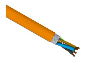
LUTZE Silflex flexible servo cable, shielded, 4 conductors (includes ground), 2 AWG, bare copper, (1) shielded 16 AWG twisted pair, PVC/Nylon conductor insulation material, brown, black, blue and green/yellow ground, TPE jacket, orange, cut to length.
