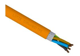
LUTZE Silflex flexible servo cable, shielded, 4 conductors (includes ground), 16 AWG, bare copper, PVC/Nylon conductor insulation material, brown, black, blue and green/yellow ground, TPE jacket, orange, cut to length.
