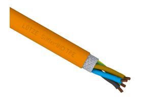
LUTZE Silflex flexible servo cable, shielded, 4 conductors (includes ground), 12 AWG, bare copper, PVC/Nylon conductor insulation material, brown, black, blue and green/yellow ground, TPE jacket, orange, cut to length.
