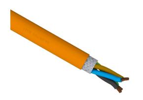
LUTZE Silflex flexible servo cable, shielded, 4 conductors (includes ground), 10 AWG, bare copper, PVC/Nylon conductor insulation material, brown, black, blue and green/yellow ground, TPE jacket, orange, cut to length.
