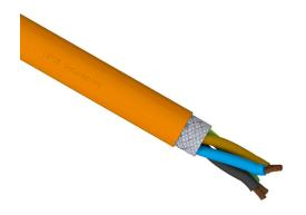
LUTZE Silflex flexible servo cable, shielded, 4 conductors (includes ground), 8 AWG, bare copper, PVC/Nylon conductor insulation material, brown, black, blue and green/yellow ground, TPE jacket, orange, cut to length.
