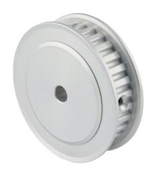
Sung-II Machinery timing pulley, aluminum, 1/5in XL pitch, 30 tooth, 1.91in pitch diameter, 1/4in bore, no hub with flanges. For use with 3/8in wide belt.
