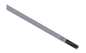
LUTZE Silflex flexible control cable, shielded, 25 conductors (includes ground), 20 AWG, bare copper, PVC/Nylon conductor insulation material, black with white numbers and green/yellow ground, PVC jacket, gray, cut to length.
