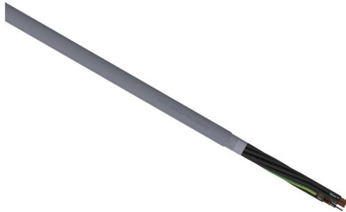
LUTZE Silflex flexible control cable, shielded, 12 conductors (includes ground), 20 AWG, bare copper, PVC/Nylon conductor insulation material, black with white numbers and green/yellow ground, PVC jacket, gray, cut to length.
