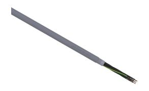
LUTZE Silflex flexible control cable, shielded, 7 conductors (includes ground), 20 AWG, bare copper, PVC/Nylon conductor insulation material, black with white numbers and green/yellow ground, PVC jacket, gray, cut to length.
