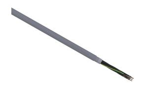
LUTZE Silflex flexible control cable, shielded, 7 conductors (includes ground), 20 AWG, bare copper, PVC/Nylon conductor insulation material, black with white numbers and green/yellow ground, PVC jacket, gray, cut to length.
