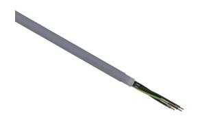
LUTZE Silflex flexible control cable, shielded, 5 conductors (includes ground), 20 AWG, bare copper, PVC/Nylon conductor insulation material, black with white numbers and green/yellow ground, PVC jacket, gray, cut to length.
