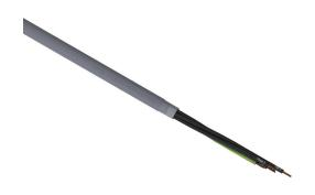
LUTZE Silflex flexible control cable, shielded, 4 conductors (includes ground), 20 AWG, bare copper, PVC/Nylon conductor insulation material, black with white numbers and green/yellow ground, PVC jacket, gray, cut to length.
