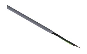
LUTZE Silflex flexible control cable, shielded, 3 conductors (includes ground), 20 AWG, bare copper, PVC/Nylon conductor insulation material, black with white numbers and green/yellow ground, PVC jacket, gray, cut to length.
