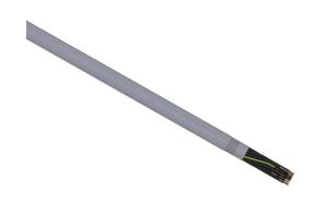
LUTZE Silflex flexible control cable, shielded, 25 conductors (includes ground), 18 AWG, bare copper, PVC/Nylon conductor insulation material, black with white numbers and green/yellow ground, PVC jacket, gray, cut to length.
