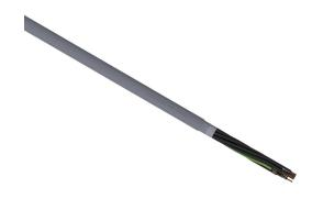
LUTZE Silflex flexible control cable, shielded, 12 conductors (includes ground), 18 AWG, bare copper, PVC/Nylon conductor insulation material, black with white numbers and green/yellow ground, PVC jacket, gray, cut to length.
