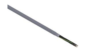
LUTZE Silflex flexible control cable, shielded, 7 conductors (includes ground), 18 AWG, bare copper, PVC/Nylon conductor insulation material, black with white numbers and green/yellow ground, PVC jacket, gray, cut to length.
