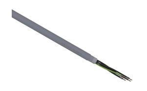
LUTZE Silflex flexible control cable, shielded, 5 conductors (includes ground), 18 AWG, bare copper, PVC/Nylon conductor insulation material, black with white numbers and green/yellow ground, PVC jacket, gray, cut to length.
