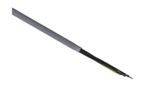
LUTZE Silflex flexible control cable, shielded, 4 conductors (includes ground), 18 AWG, bare copper, PVC/Nylon conductor insulation material, black with white numbers and green/yellow ground, PVC jacket, gray, cut to length.
