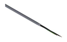
LUTZE Silflex flexible control cable, shielded, 3 conductors (includes ground), 18 AWG, bare copper, PVC/Nylon conductor insulation material, black with white numbers and green/yellow ground, PVC jacket, gray, cut to length.
