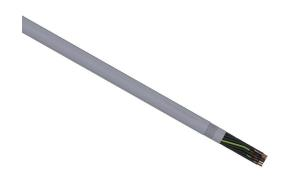
LUTZE Silflex flexible control cable, shielded, 25 conductors (includes ground), 16 AWG, bare copper, PVC/Nylon conductor insulation material, black with white numbers and green/yellow ground, PVC jacket, gray, cut to length.
