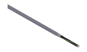
LUTZE Silflex flexible control cable, shielded, 7 conductors (includes ground), 16 AWG, bare copper, PVC/Nylon conductor insulation material, black with white numbers and green/yellow ground, PVC jacket, gray, cut to length.
