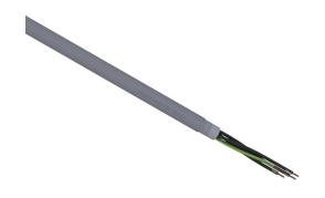
LUTZE Silflex flexible control cable, shielded, 5 conductors (includes ground), 16 AWG, bare copper, PVC/Nylon conductor insulation material, black with white numbers and green/yellow ground, PVC jacket, gray, cut to length.
