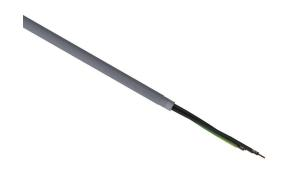
LUTZE Silflex flexible control cable, shielded, 3 conductors (includes ground), 16 AWG, bare copper, PVC/Nylon conductor insulation material, black with white numbers and green/yellow ground, PVC jacket, gray, cut to length.
