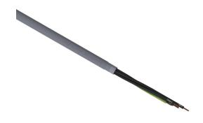
LUTZE Silflex flexible control cable, shielded, 4 conductors (includes ground), 14 AWG, bare copper, PVC/Nylon conductor insulation material, black with white numbers and green/yellow ground, PVC jacket, gray, cut to length.
