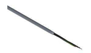
LUTZE Silflex flexible control cable, shielded, 3 conductors (includes ground), 14 AWG, bare copper, PVC/Nylon conductor insulation material, black with white numbers and green/yellow ground, PVC jacket, gray, cut to length.
