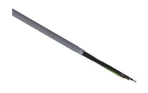
LUTZE Silflex flexible control cable, shielded, 4 conductors (includes ground), 12 AWG, bare copper, PVC/Nylon conductor insulation material, black with white numbers and green/yellow ground, PVC jacket, gray, cut to length.
