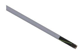
LUTZE Silflex flexible control cable, unshielded, 25 conductors (includes ground), 20 AWG, bare copper, PVC/Nylon conductor insulation material, black with white numbers and green/yellow ground, PVC jacket, gray, cut to length.
