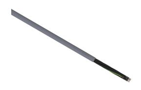
LUTZE Silflex flexible control cable, unshielded, 12 conductors (includes ground), 20 AWG, bare copper, PVC/Nylon conductor insulation material, black with white numbers and green/yellow ground, PVC jacket, gray, cut to length.
