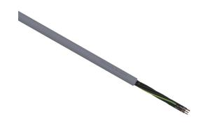
LUTZE Silflex flexible control cable, unshielded, 7 conductors (includes ground), 20 AWG, bare copper, PVC/Nylon conductor insulation material, black with white numbers and green/yellow ground, PVC jacket, gray, cut to length.
