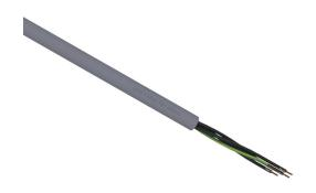
LUTZE Silflex flexible control cable, unshielded, 5 conductors (includes ground), 20 AWG, bare copper, PVC/Nylon conductor insulation material, black with white numbers and green/yellow ground, PVC jacket, gray, cut to length.
