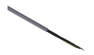
LUTZE Silflex flexible control cable, unshielded, 4 conductors (includes ground), 20 AWG, bare copper, PVC/Nylon conductor insulation material, black with white numbers and green/yellow ground, PVC jacket, gray, cut to length.
