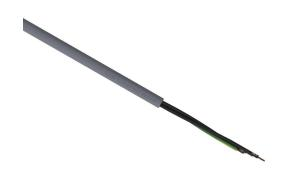
LUTZE Silflex flexible control cable, unshielded, 3 conductors (includes ground), 20 AWG, bare copper, PVC/Nylon conductor insulation material, black with white numbers and green/yellow ground, PVC jacket, gray, cut to length.
