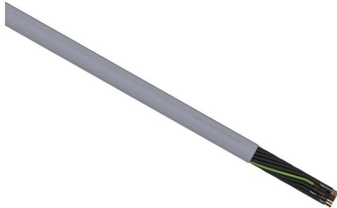
LUTZE Silflex flexible control cable, unshielded, 25 conductors (includes ground), 18 AWG, bare copper, PVC/Nylon conductor insulation material, black with white numbers and green/yellow ground, PVC jacket, gray, cut to length.
