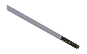
LUTZE Silflex flexible control cable, unshielded, 25 conductors (includes ground), 18 AWG, bare copper, PVC/Nylon conductor insulation material, black with white numbers and green/yellow ground, PVC jacket, gray, cut to length.
