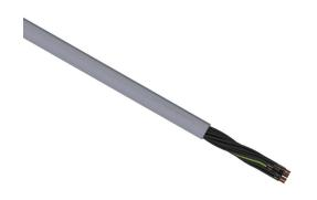
LUTZE Silflex flexible control cable, unshielded, 18 conductors (includes ground), 18 AWG, bare copper, PVC/Nylon conductor insulation material, black with white numbers and green/yellow ground, PVC jacket, gray, cut to length.
