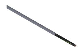
LUTZE Silflex flexible control cable, unshielded, 12 conductors (includes ground), 18 AWG, bare copper, PVC/Nylon conductor insulation material, black with white numbers and green/yellow ground, PVC jacket, gray, cut to length.
