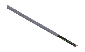
LUTZE Silflex flexible control cable, unshielded, 9 conductors (includes ground), 18 AWG, bare copper, PVC/Nylon conductor insulation material, black with white numbers and green/yellow ground, PVC jacket, gray, cut to length.
