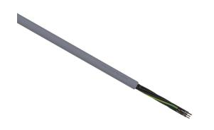
LUTZE Silflex flexible control cable, unshielded, 7 conductors (includes ground), 18 AWG, bare copper, PVC/Nylon conductor insulation material, black with white numbers and green/yellow ground, PVC jacket, gray, cut to length.
