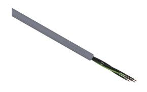
LUTZE Silflex flexible control cable, unshielded, 5 conductors (includes ground), 18 AWG, bare copper, PVC/Nylon conductor insulation material, black with white numbers and green/yellow ground, PVC jacket, gray, cut to length.
