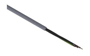
LUTZE Silflex flexible control cable, unshielded, 4 conductors (includes ground), 18 AWG, bare copper, PVC/Nylon conductor insulation material, black with white numbers and green/yellow ground, PVC jacket, gray, cut to length.
