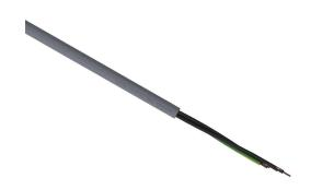
LUTZE Silflex flexible control cable, unshielded, 3 conductors (includes ground), 18 AWG, bare copper, PVC/Nylon conductor insulation material, black with white numbers and green/yellow ground, PVC jacket, gray, cut to length.
