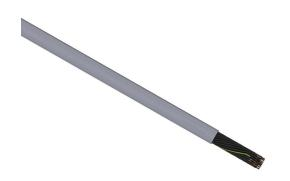
LUTZE Silflex flexible control cable, unshielded, 41 conductors (includes ground), 16 AWG, bare copper, PVC/Nylon conductor insulation material, black with white numbers and green/yellow ground, PVC jacket, gray, cut to length.
