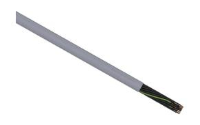
LUTZE Silflex flexible control cable, unshielded, 25 conductors (includes ground), 16 AWG, bare copper, PVC/Nylon conductor insulation material, black with white numbers and green/yellow ground, PVC jacket, gray, cut to length.
