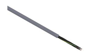
LUTZE Silflex flexible control cable, unshielded, 7 conductors (includes ground), 16 AWG, bare copper, PVC/Nylon conductor insulation material, black with white numbers and green/yellow ground, PVC jacket, gray, cut to length.
