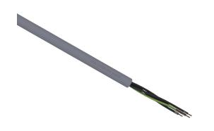
LUTZE Silflex flexible control cable, unshielded, 5 conductors (includes ground), 16 AWG, bare copper, PVC/Nylon conductor insulation material, black with white numbers and green/yellow ground, PVC jacket, gray, cut to length.
