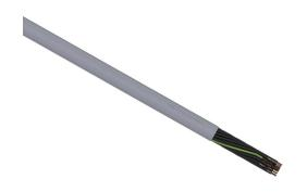
LUTZE Silflex flexible control cable, unshielded, 25 conductors (includes ground), 14 AWG, bare copper, PVC/Nylon conductor insulation material, black with white numbers and green/yellow ground, PVC jacket, gray, cut to length.
