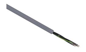
LUTZE Silflex flexible control cable, unshielded, 5 conductors (includes ground), 14 AWG, bare copper, PVC/Nylon conductor insulation material, black with white numbers and green/yellow ground, PVC jacket, gray, cut to length.
