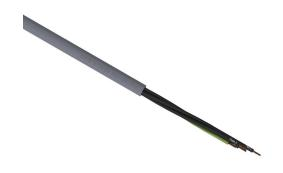
LUTZE Silflex flexible control cable, unshielded, 4 conductors (includes ground), 14 AWG, bare copper, PVC/Nylon conductor insulation material, black with white numbers and green/yellow ground, PVC jacket, gray, cut to length.
