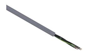
LUTZE Silflex flexible control cable, unshielded, 5 conductors (includes ground), 12 AWG, bare copper, PVC/Nylon conductor insulation material, black with white numbers and green/yellow ground, PVC jacket, gray, cut to length.
